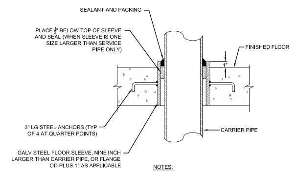
THE CONTRACTOR SHALL CORE EXISTING FLOORS AND SEAL AS SHOWN. STEEL SLEEVE TO BE ELIMINATED IN EXISTING CONSTRUCTION.
